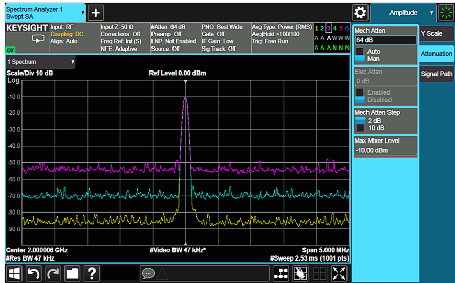
Figure 5-1. In modern signal analyzers, reference levels remain constant when you change input attenuation
