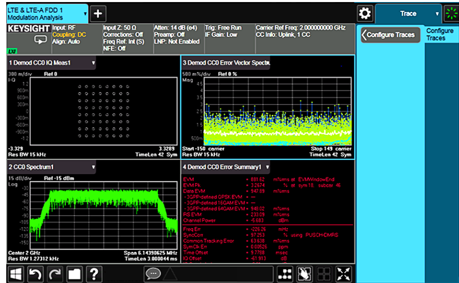
Figure 8-6. EVM measurement of LTE FDD downlink signal
